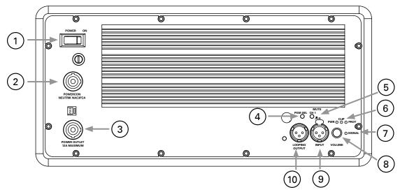
1. **Power Switch** – Turns unit power ON or OFF.
