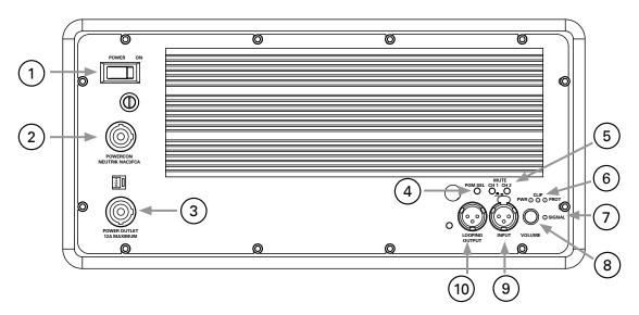
1. **Power Switch** – Turns unit power ON or OFF.
