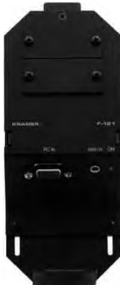
Figure 1: The F-121 XGA / Audio Line Driver Mounting Box
