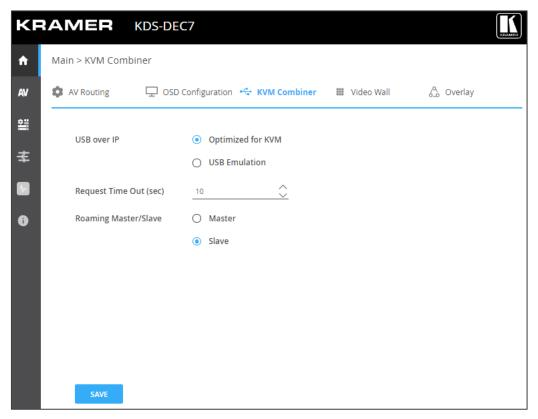
Figure 59: Defining the Master Decoder for KVM Roaming
