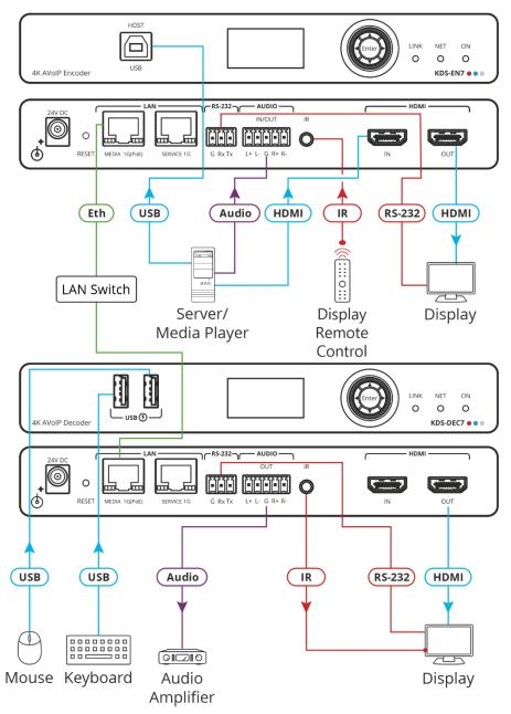
Figure 3: Connecting the KDS-EN7 and KDS-DEC7
