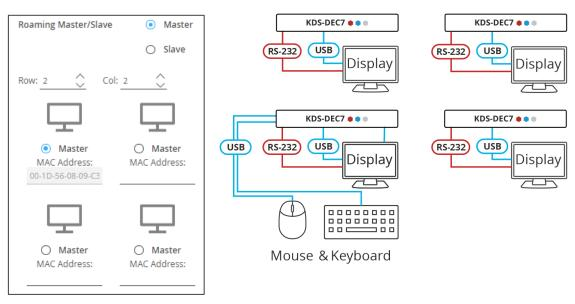
Figure 60: Setting the decoder configuration
