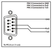
Figure 14: RS-232 PINOUT Connection
