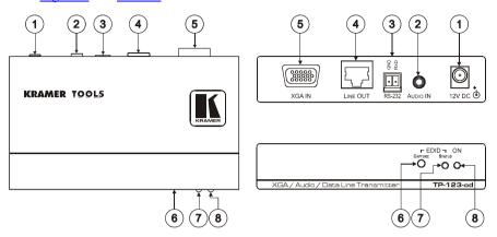
Figure 7: TP-123-od XGA / Audio / Data Line Transmitter
