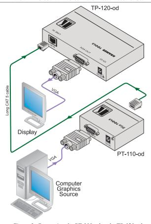
Figure 3: Connecting the PT-110-od to the TP-120-od
