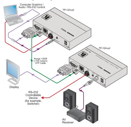
Figure 9: Connecting the TP-123-od and the TP-124-od
