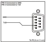
Figure 10: RS-232 PINOUT Connection
