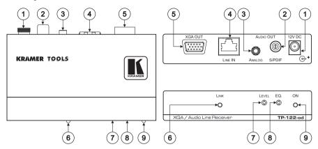
Figure 5: TP-122-od XGA / Audio Line Receiver (Topside)
