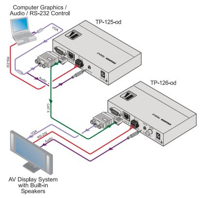
Figure 13: Connecting the TP-125-od and the TP-126-od
