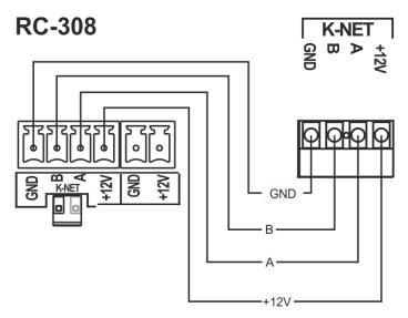
Figure 9: K-NET PINOUT Connection
