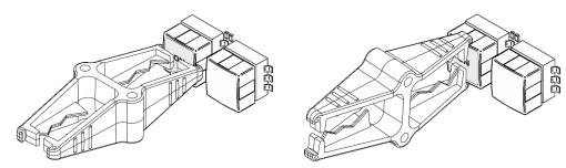
Figure 6: Removing the Button Cap
