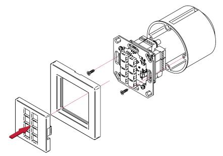
Figure 11: Installing the RC-308 EU/UK Version
