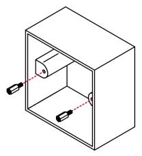
Figure 12: Using Spacers for BS-EN 60670-1 Junction Box
