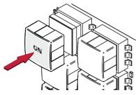
Figure 5: Attaching the Button
