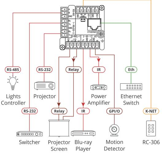
Figure 7: Connecting to the RC-308 Rear Panel
