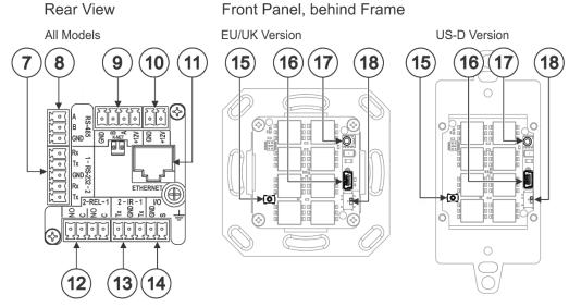
Figure 3: Ethernet and K-NET Control Keypad Rear View
