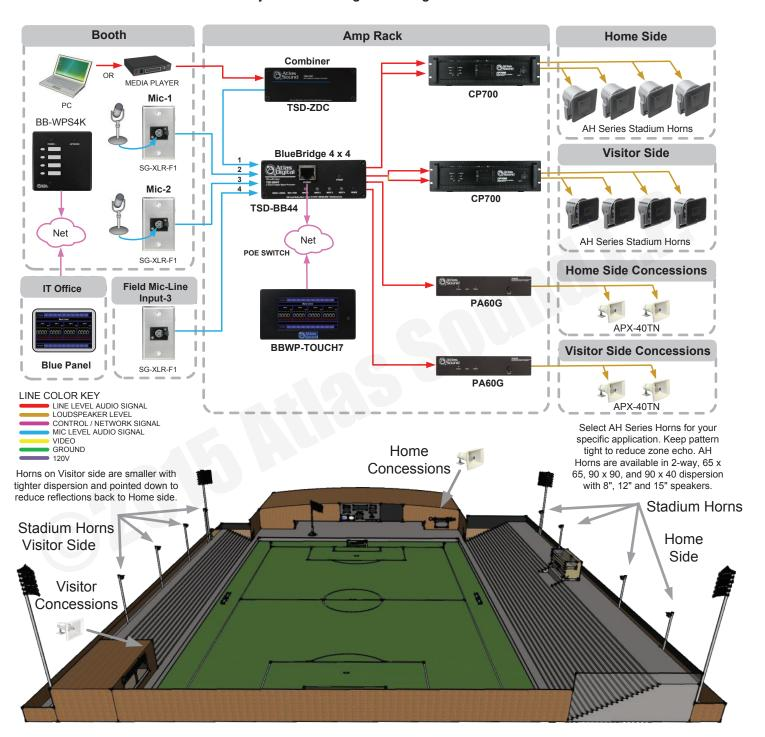
This is a design concept and is not meant to be a fully engineered system design. Contact Atlas Sound for system design help.
