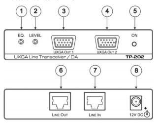
Figure 1: TP-202 UXGA Line Transceiver/DA
