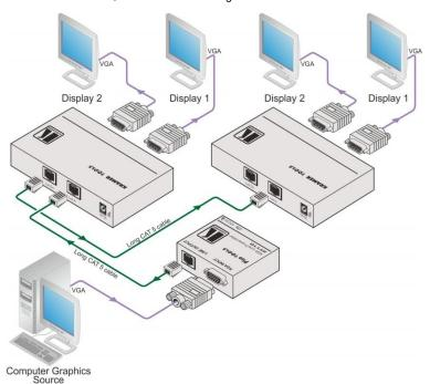
Figure 3: Connecting the TP-202 UXGA Line Transceiver/DA
