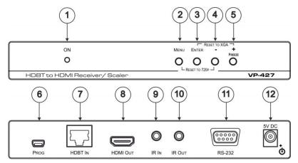
Figure 1: VP-427 HDBaseT to HDMI Receiver/Scaler
