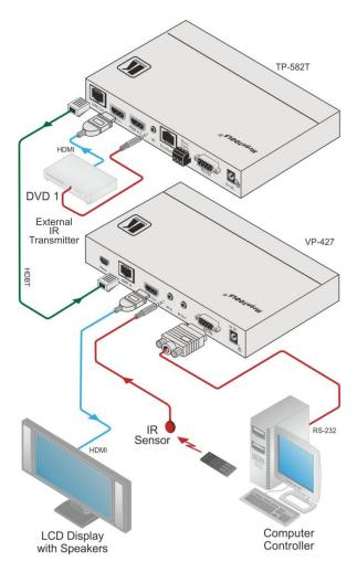
Figure 2: Connecting the VP-427 HDBaseT to HDMI Receiver/Scaler
