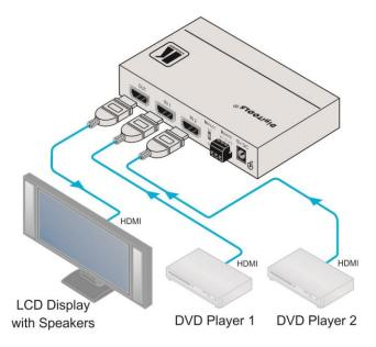
Figure 2: VS-211H Connections
