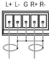
Figure 7: Unbalanced Stereo Audio Input Connection
