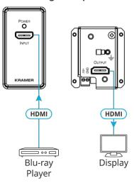
The WP-3H2 / W-3H2 input is connected via a male-to-male HDMI cable (not provided) to an HDMI source, such as a 4K UHD Blu-ray player.
